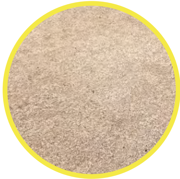
INFORMAL PATHWAY COMPACTED LIMESTONE 5% CONCRETE MIX
