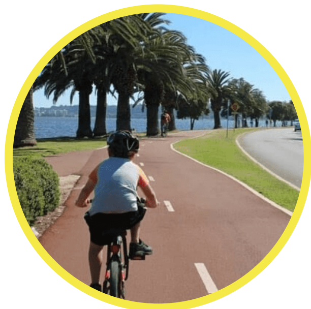
RED ASPHALT TRAFFICABLE DUAL USE PATH PRIMARYLY FOR PEDESTRIAN USE (ALLOWS FOR MAINTENANCE AC- CESS)
