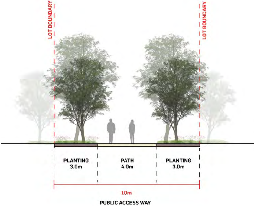
Figure 11 - Cross Section with Landscape Treatment
