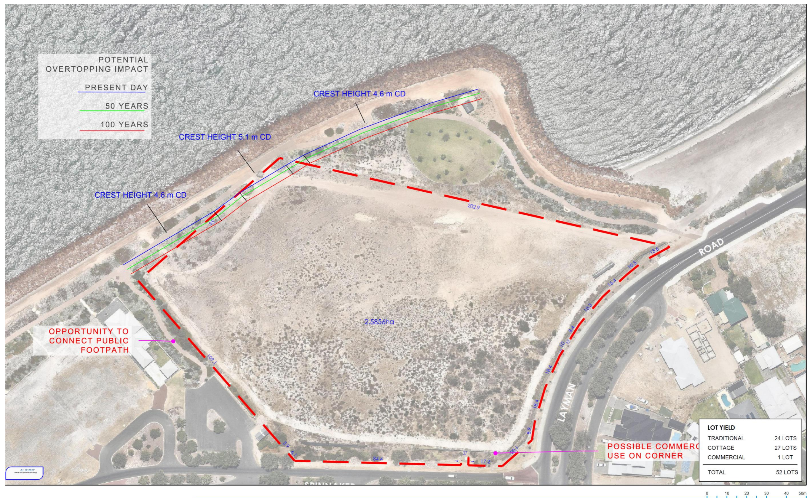
Figure 2.2 Potential Extent of Wave Overtopping Impact on Building Structural Elements
