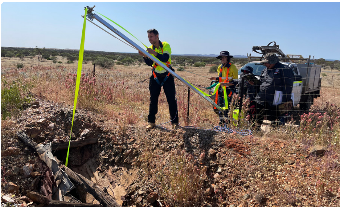
Down-hole LiDAR scanning of abandoned shaft feature.
