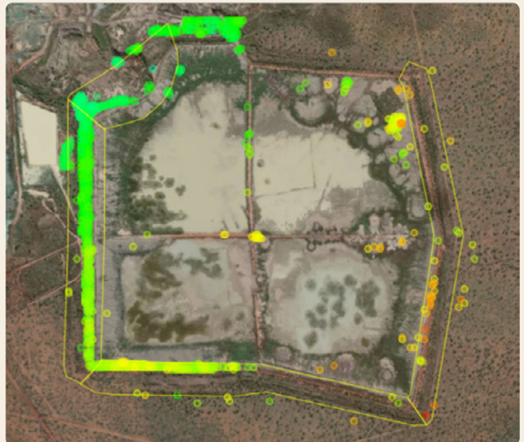
Ellendale TSF1D showing wall variance over the duration of several months.
