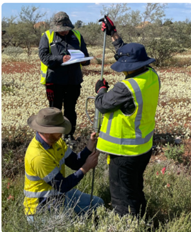
Left: Yalgoo phase 1 stage 2 geotechnical investigation completed: testing relative soil density. Right: Testing shaft base stability and surrounding soil conditions.
