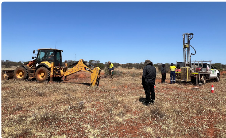
Left: Yalgoo phase 1 stage 2 geotechnical investigation completed: testing relative soil density. Right: Testing shaft base stability and surrounding soil conditions.
