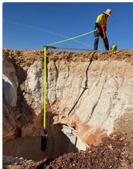
Cue phase 1 stage 1 geotechnical assessment in progress. Left: Open abandoned mine shaft with erosion evident around original timbers. Right: Down-hole LiDAR scanning of abandoned mine feature with eroding collar.
