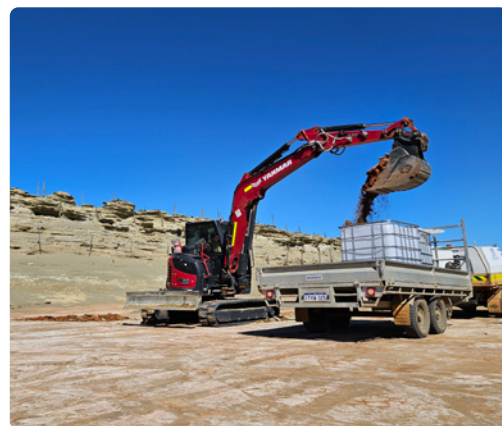
Preparing bulk samples of Elverdton tailings material for modelling.
