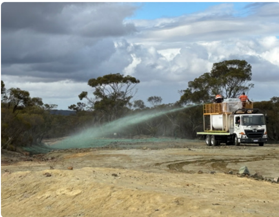
Dust suppressant trial over the deposition fan. Left: Dust suppressant application. Right: View of trial area.
