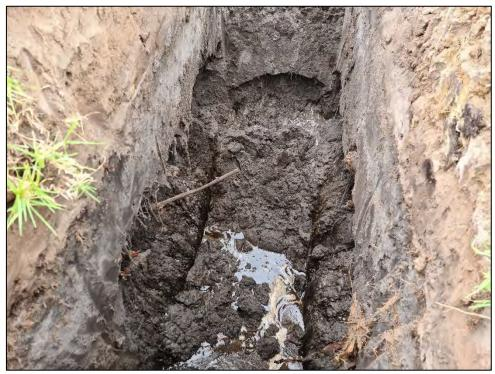
Figure 88: Test Pit 44 Soil Profile
