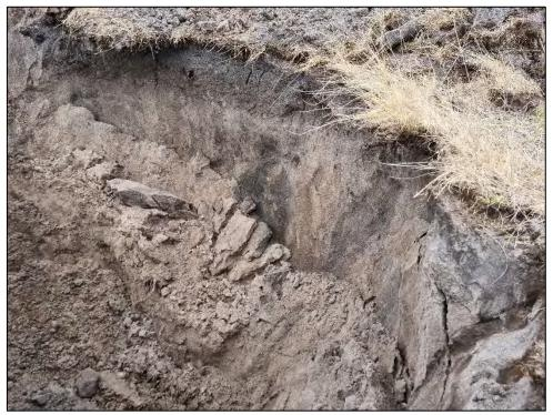
Figure 44: Test Pit 22 Soil Profile
