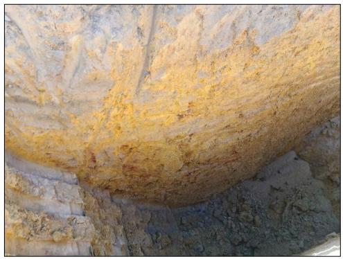
Figure 24: Test Pit 12 Soil Profile
