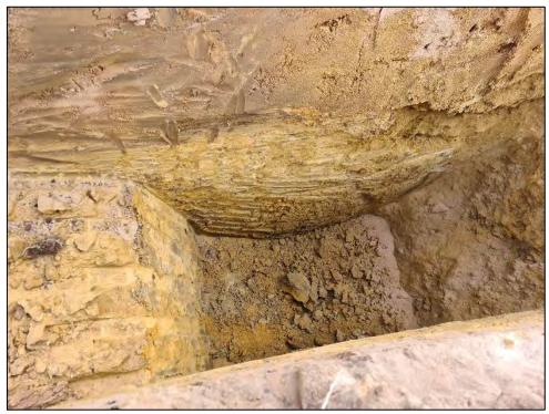
Figure 116: Test Pit 58 Soil Profile
