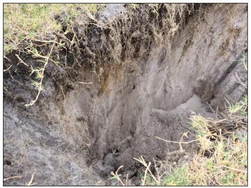
Figure 58: Test Pit 29 Soil Profile
