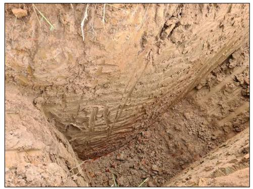
Figure 72: Test Pit 36 Soil Profile
