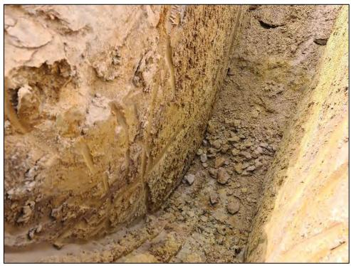
Figure 52: Test Pit 26 Soil Profile
