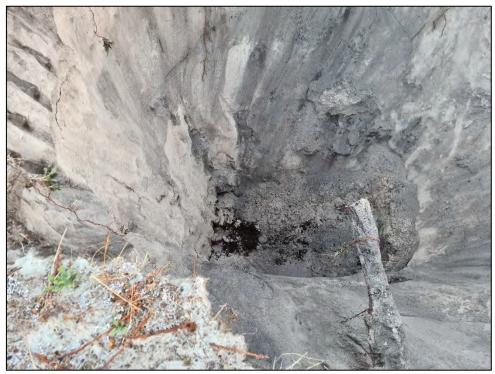
Figure 108: Test Pit 54 Soil Profile
