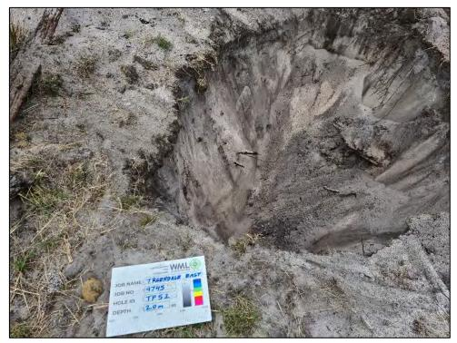
Figure 103: Test Pit 52 Excavation
