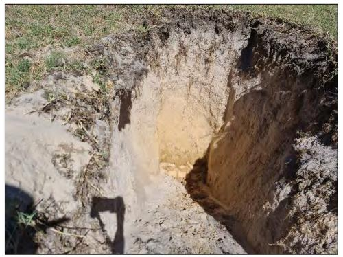
Figure 130: Test Pit 65 Soil Profile
