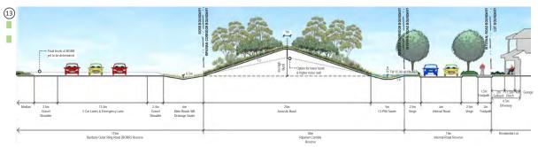
ACCESS STREET D, ADJACENT BIORETENTION SWALE/ LANDSCAPED BUFFER & BORR (13m) SCALE 1:500 @ A4  $\,$
