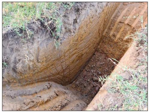
Figure 2: Test Pit 1 Soil Profile
