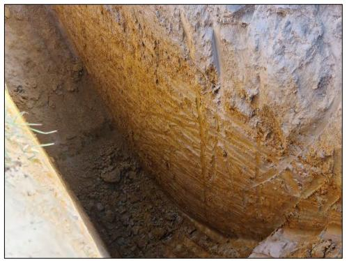
Figure 10: Test Pit 5 Soil Profile
