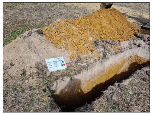
Figure 9: Test Pit 5 Excavation Site and Arisings
