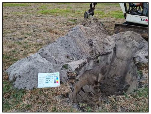
Figure 31: Test Pit 16 Excavation and Arisings
