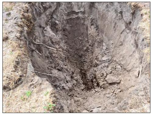
Figure 118: Test Pit 59 Soil Profile
