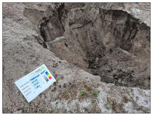
Figure 101: Test Pit 51 Excavation
