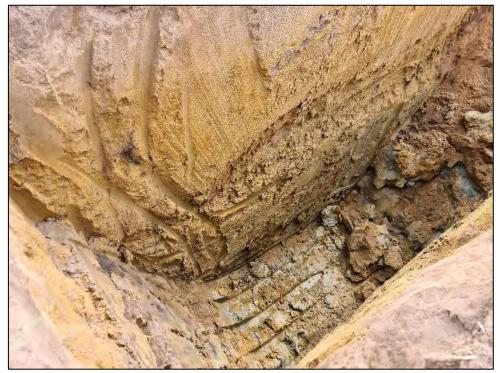
Figure 48: Test Pit 24 Soil Profile
