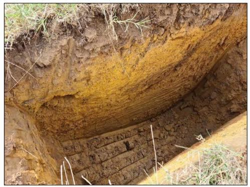
Figure 20: Test Pit 10 Soil Profile
