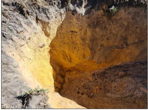
Figure 138: Test Pit 69 Soil Profile
