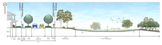
ACCESS STREET D, ADJACENT UPSTREAM DRAINAGE (15m) SCALE 1:500 @ A4  $\,$
