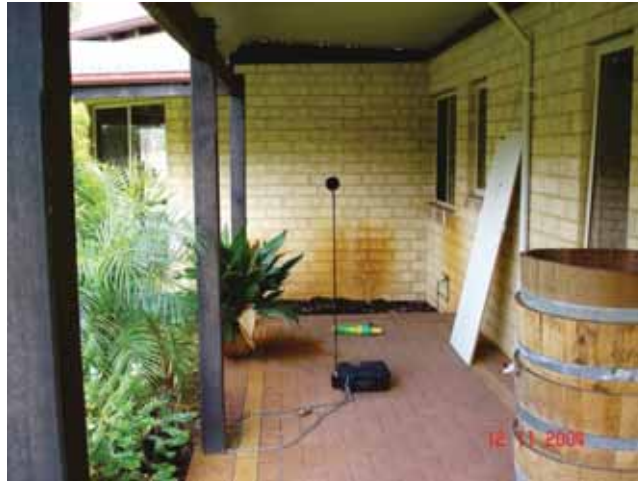
Figure 3.1 – Automatic Noise Data Logger
