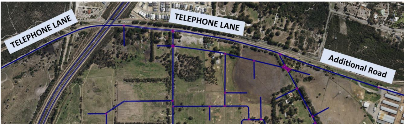
Figure 5-5: Overview of Connections to Telephone Lane
