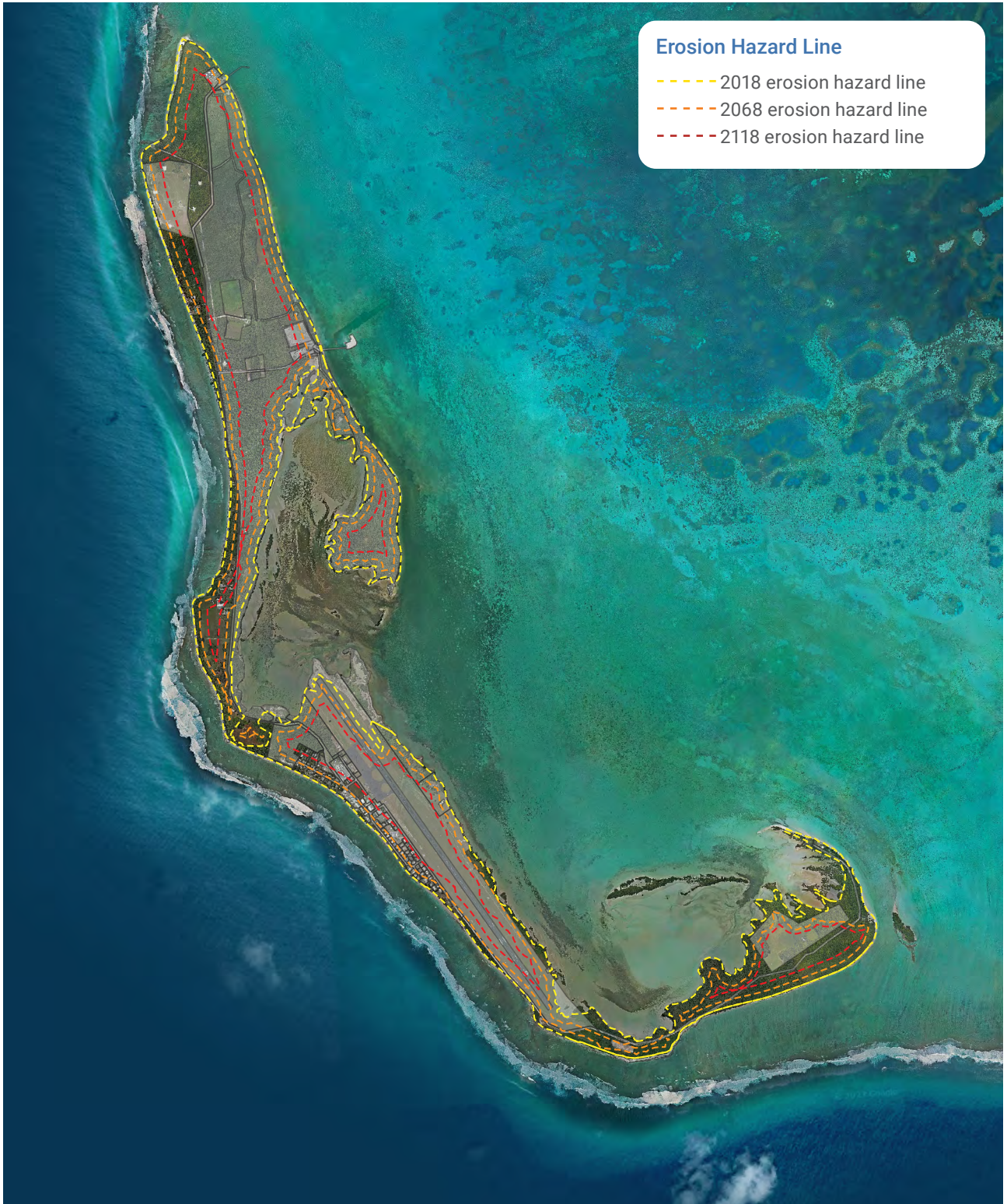
Figure 44: West Island erosion allowance
