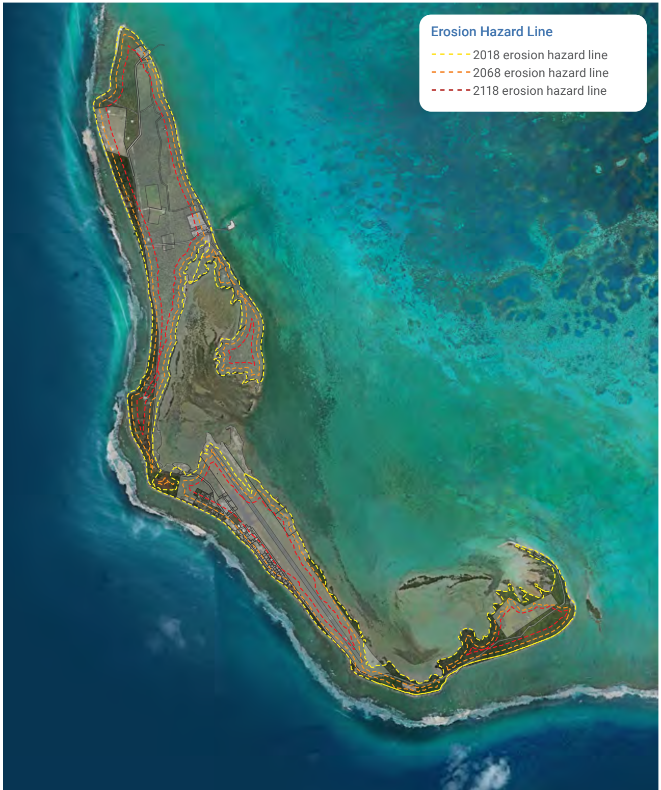
Figure 44: West Island erosion allowance
