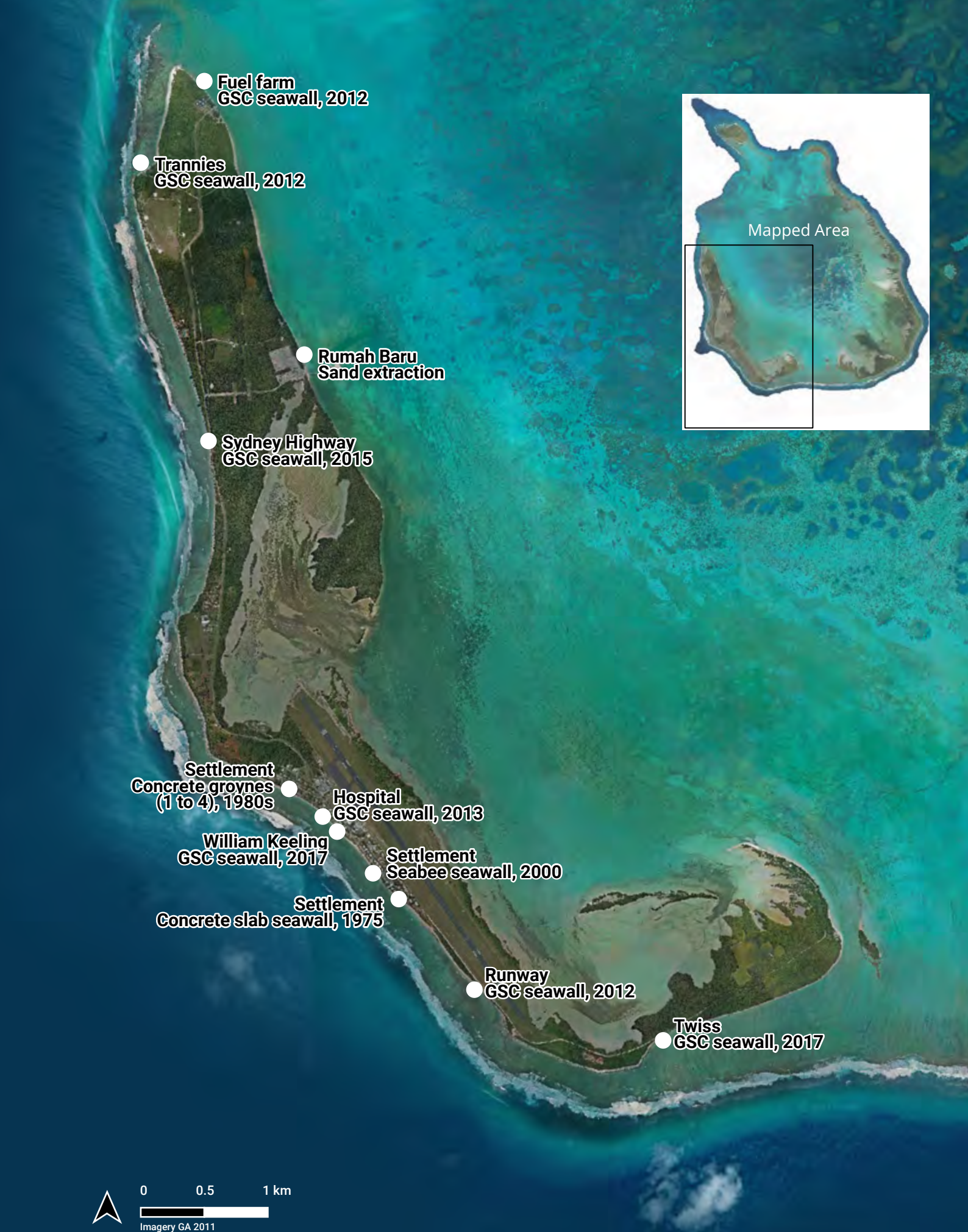
Figure 22: Existing controls on West Island
