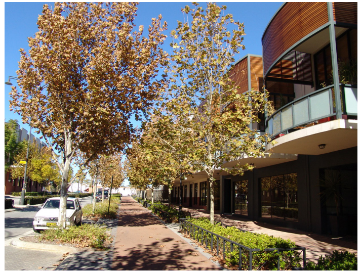
Setbacks enable tree planting which can provide a buffer to adjacent developments, through minimising overlooking and improving the outlook from upper level apartments.
