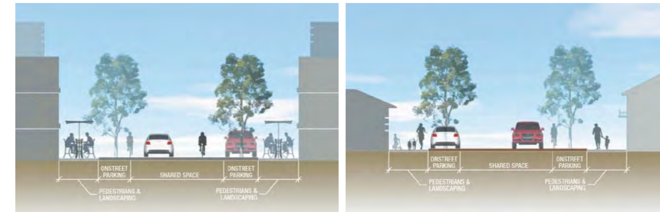
Figure 19 Indicative cross section – Local Access ways
