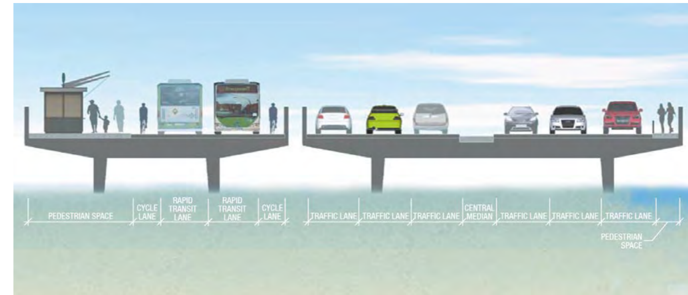
Figure 15 Indicative cross section – Canning River Bridge
