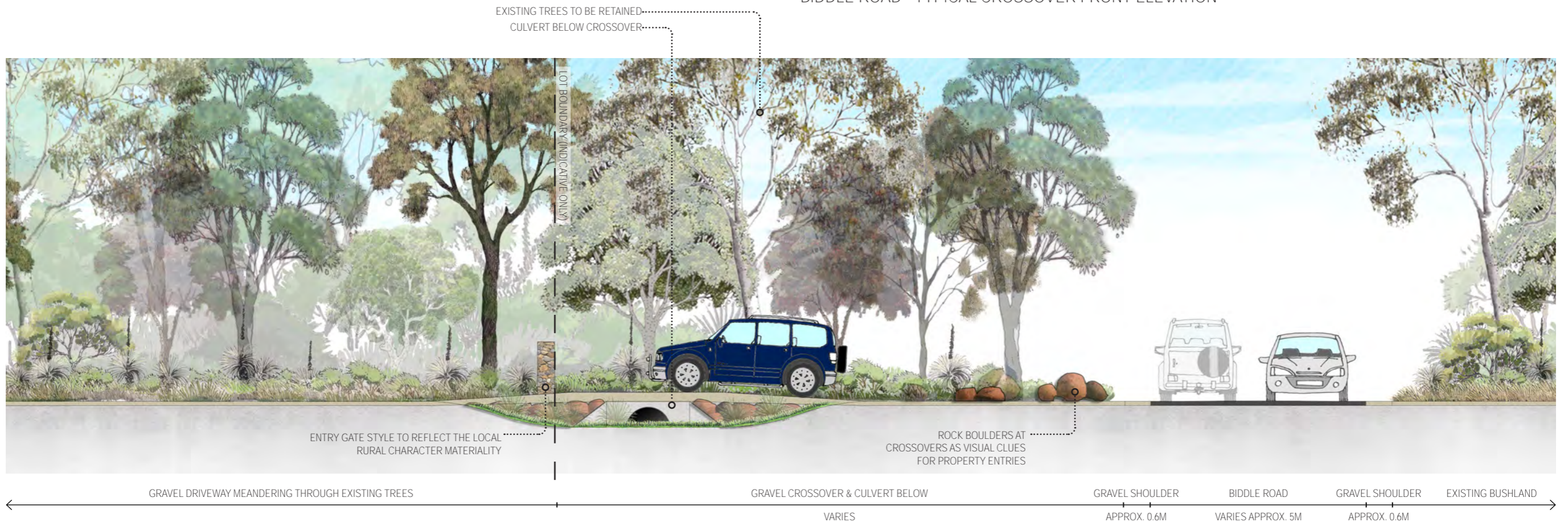
BIDDLE ROAD - TYPICAL CROSSOVER FRONT ELEVATION
