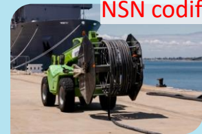
RAPID REEL™ Deployment, retrieval and storage system expediting shore power & flat fuel hose handling.
