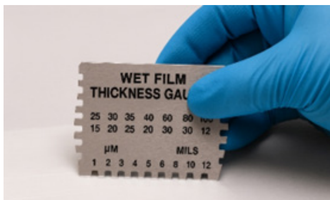
Figure 6: Wet film thickness gauge used to measure film thickness of applied material.
