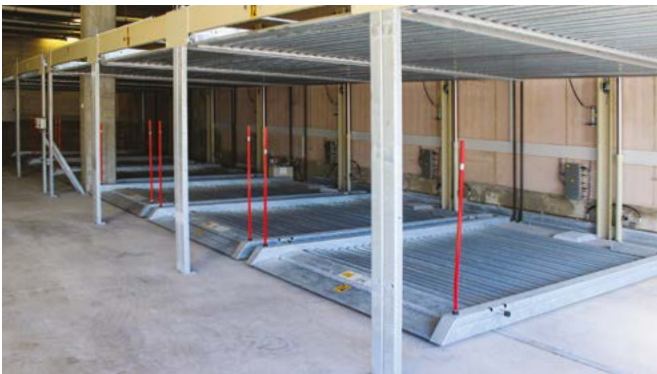
Photo 3.9d Car stackers can provide a space-efficient solution.
