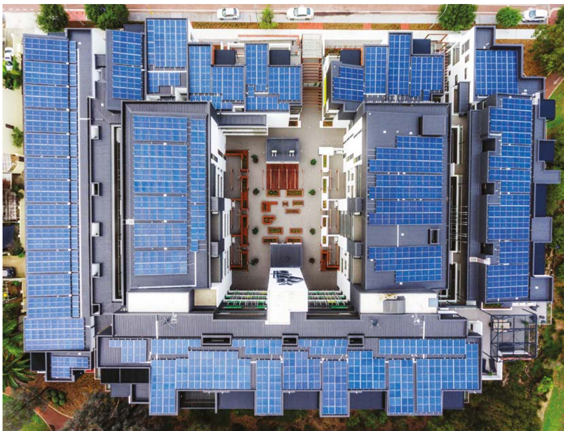
Photo 4.15a This apartment development fully utilises the roof with the installation of photo-voltaic arrays to supplement the power consumption of the dwelling units. (PC)
