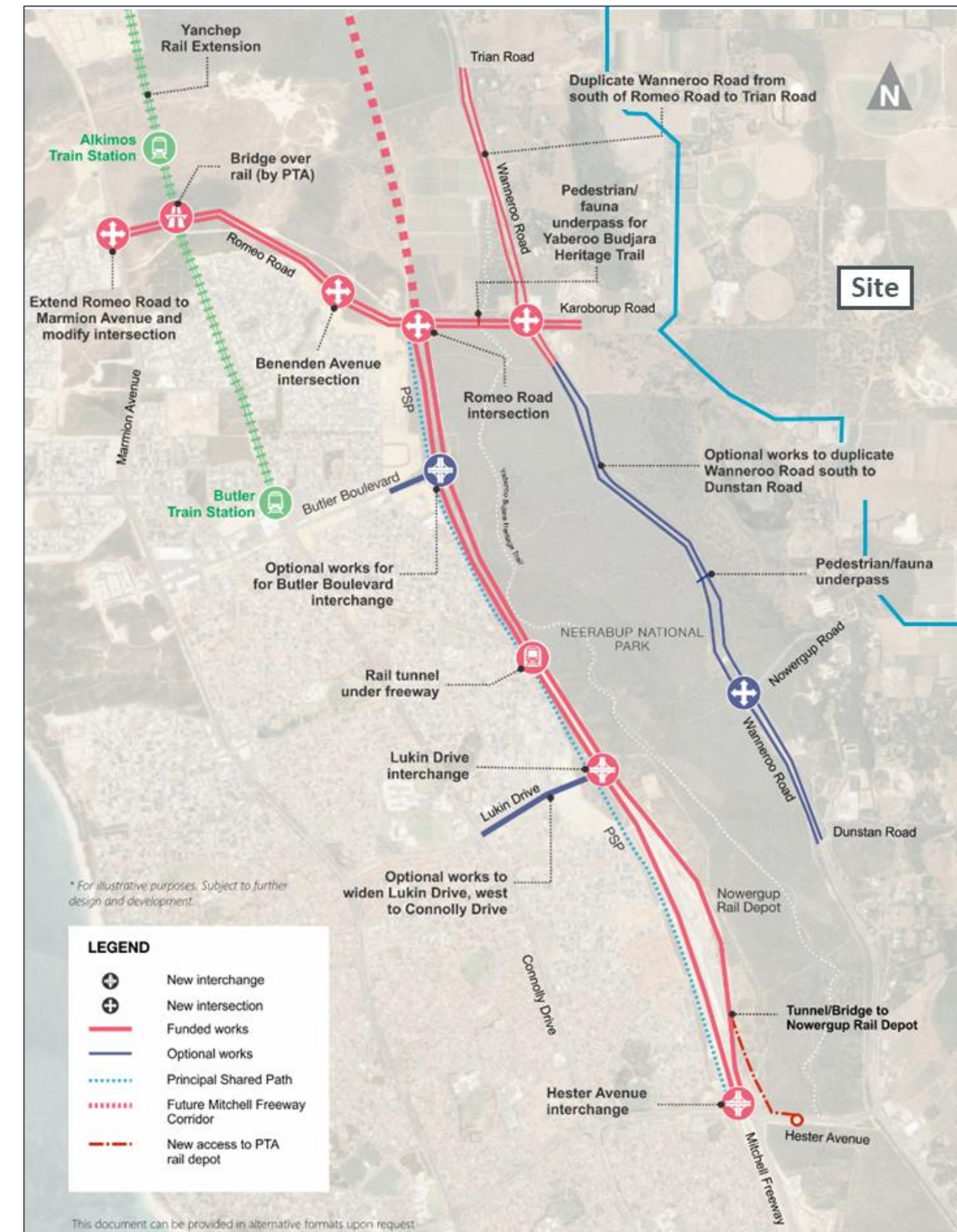
Figure 5-2: Mitchell Freeway Extension Project Extent
