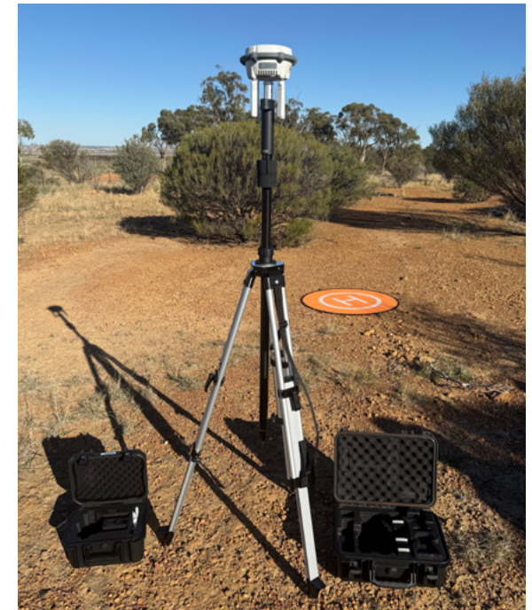
Real-Time Kinematic base station for advanced satellite positioning.
