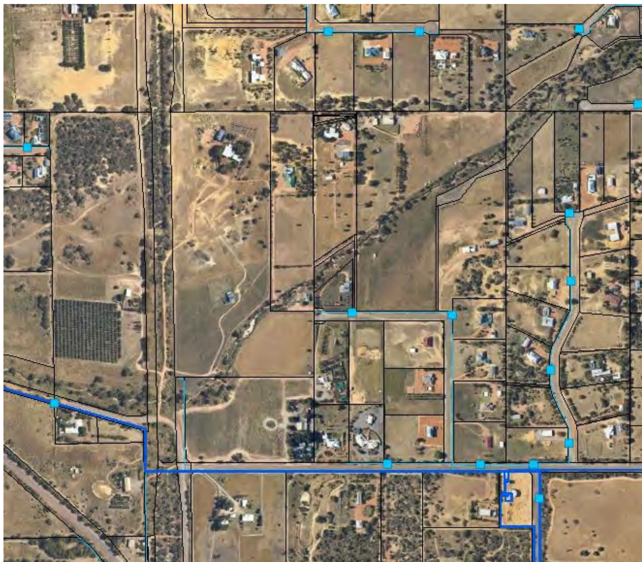
Plate 1: Existing Water Corporation pipe and hydrants
